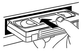
2 Insert the cassette into the cassette slot with the label facing towards you. The window must be facing upwards.
